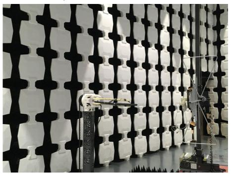
Description: Substitution Antenna for ERP Test
