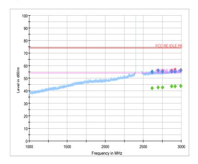
Fig.46 Radiated emission:  $\pi/4$  DQPSK, Ch0, 1GHz~3GHz
