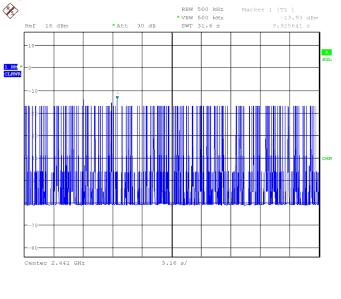
Fig.70 Number of Transmissions Measurement: Ch39, Packet 3-DH3
