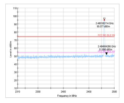
Fig.44 Radiated emission (Power): GFSK, high channel
