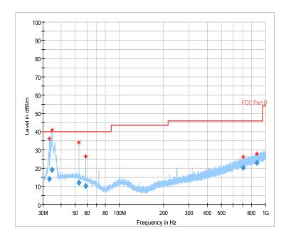
Fig.40 Radiated emission: GFSK, Ch0, 30MHz~1GHz
