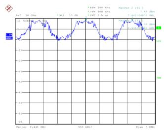
Fig.82 Carrier separation measurement: GFSK, Ch39
