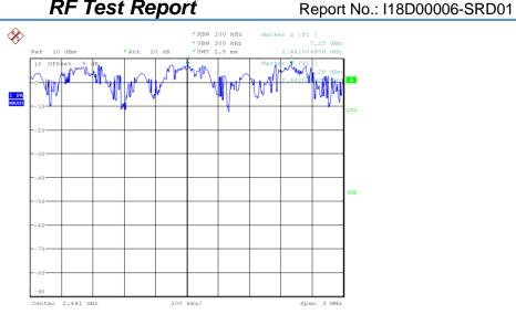
Fig.84 Carrier separation measurement: 8DPSK, Ch39
