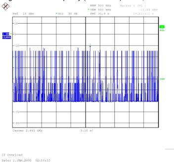
Fig.72 Number of Transmissions Measurement: Ch39, Packet 3-DH5
