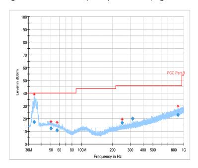
Fig.50 Radiated emission: 8DPSK, Ch0, 30MHz~1GHz
