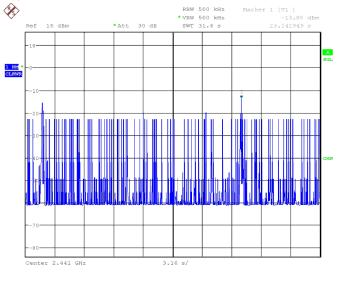
Fig.66 Number of Transmissions Measurement: Ch39, Packet 2-DH5
