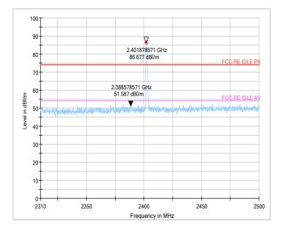
Fig.43 Radiated emission (Power): GFSK, low channel
