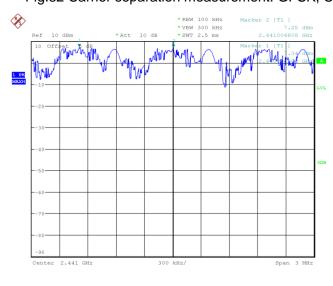
Fig.83 Carrier separation measurement: π/4 DQPSK, Ch39
