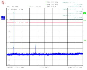
Fig.39 Conducted spurious emission: 8DPSK, Ch78, 30MHz~26GHz
