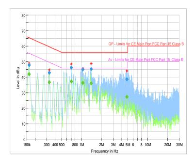
Fig.91 AC Powerline Conducted Emission
