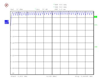
Fig.85 Number of hopping frequency: GFSK, Ch0~39
