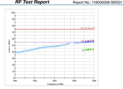
Fig.51 Radiated emission: 8DPSK, Ch0, 1GHz~3GHz
