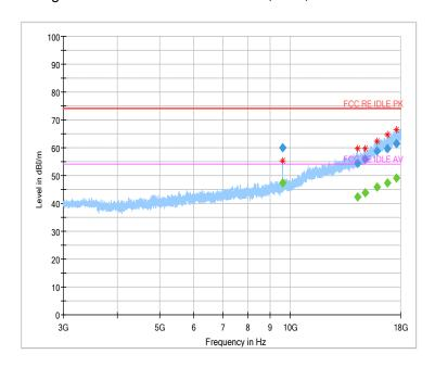
Fig.52 Radiated emission: 8DPSK, Ch0, 3GHz~18GHz
