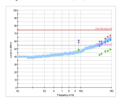
Fig.42 Radiated emission: GFSK, Ch0, 3GHz~18GHz
