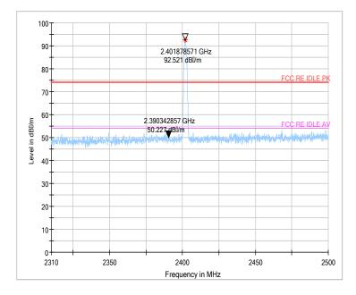
Fig.53 Radiated emission (Power): 8DPSK, low channel
