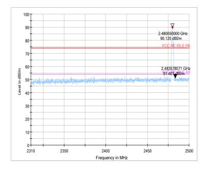
Fig.54 Radiated emission (Power): 8DPSK, high channel
