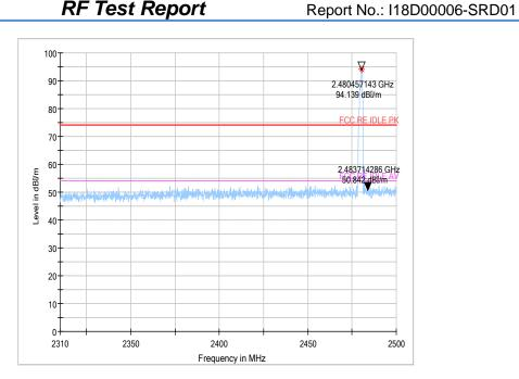
Fig.49 Radiated emission (Power): π/4 DQPSK, high channel
