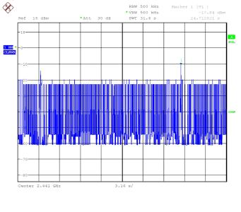
Fig.62 Number of Transmissions Measurement: Ch39, Packet 2-DH1
