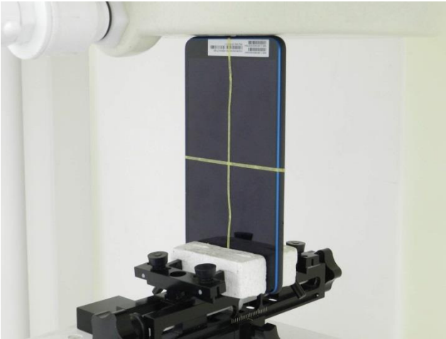
Edge3, Test Separation 0 mm
