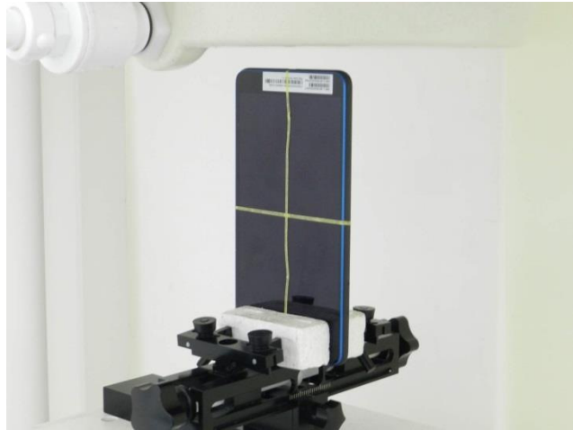
Edge3, Test Separation 14 mm
