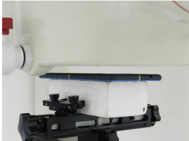
Bottom Face, Test Separation 11 mm
