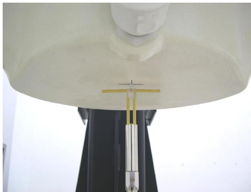
Picture 8.2 Photo of Dipole Setup
