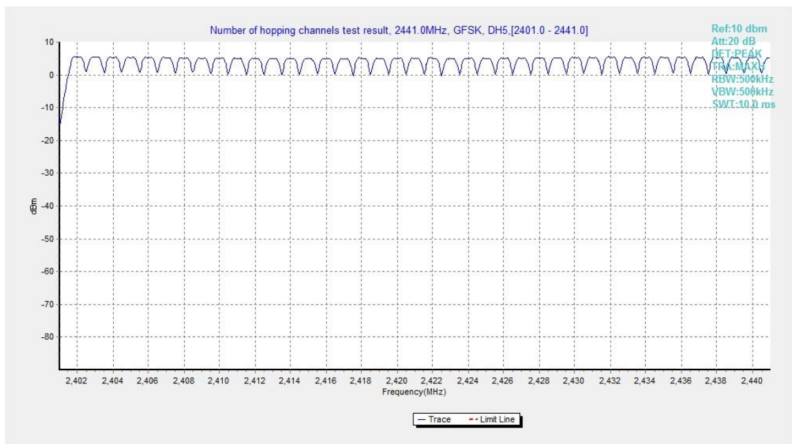
Fig.94. Number of hopping frequencies: GFSK, Channel 0 - 39
