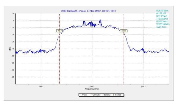
Fig.88. 20dB Bandwidth: 8DPSK, Channel 0
