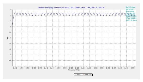
Fig.94. Number of hopping frequencies: GFSK, Channel 0 - 39
