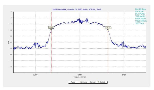
Fig.90. 20dB Bandwidth: 8DPSK, Channel 78
