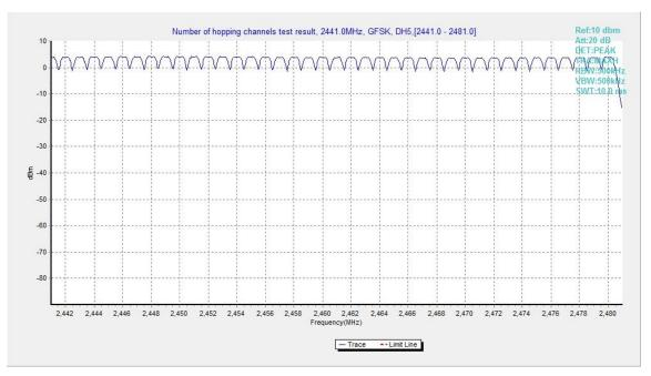
Fig.95. Number of hopping frequencies: GFSK, Channel 40 - 78
