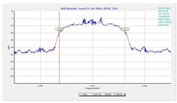
Fig.89. 20dB Bandwidth: 8DPSK, Channel 39
