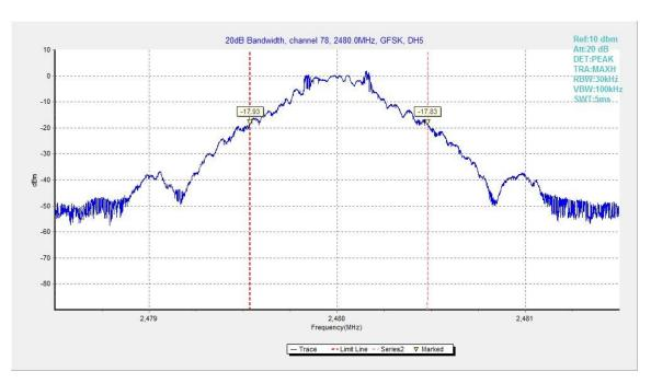
Fig.84. 20dB Bandwidth: GFSK, Channel 78
