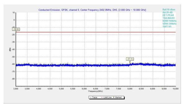
Fig.16. Conducted spurious emission: GFSK, Channel 0, 3GHz - 10GHz
