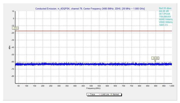
Fig.39. Conducted spurious emission: π/4 DQPSK, Channel 78, 30MHz - 1GHz
