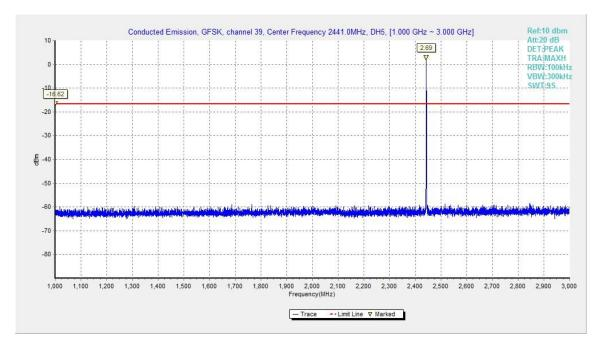
Fig.20. Conducted spurious emission: GFSK, Channel 39, 1GHz – 3GHz
