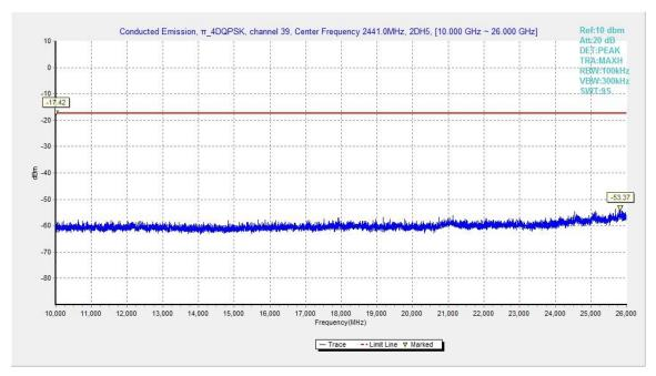
Fig.37. Conducted spurious emission: π/4 DQPSK, Channel 39, 10GHz – 26GHz
