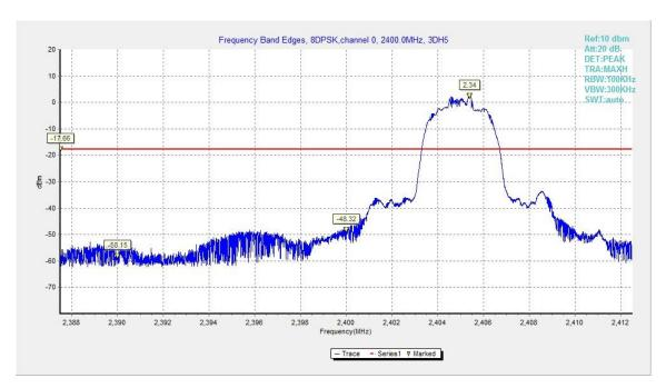
Fig.9. Frequency Band Edges: 8DPSK, Channel 0, Hopping Off
