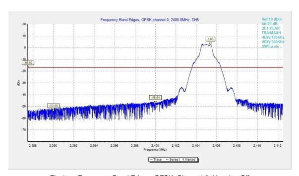
Fig.1. Frequency Band Edges: GFSK, Channel 0, Hopping Off
