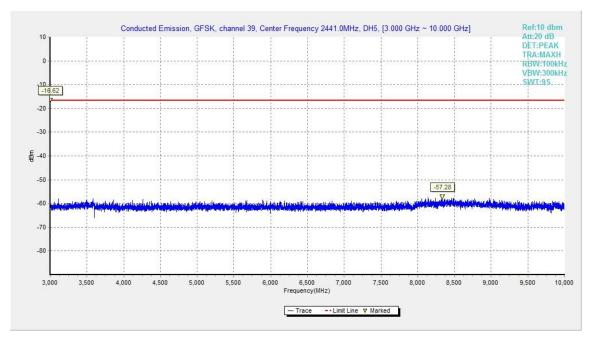
Fig.21. Conducted spurious emission: GFSK, Channel 39, 3GHz - 10GHz
