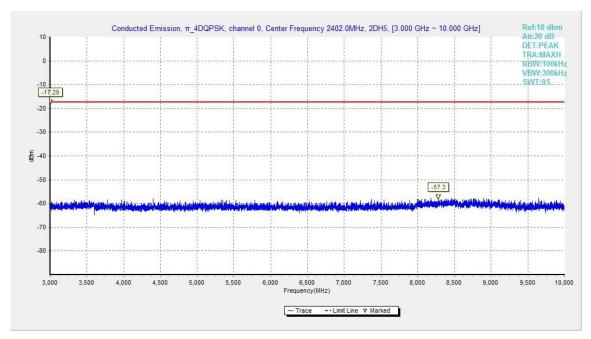
Fig.31. Conducted spurious emission: π/4 DQPSK, Channel 0, 3GHz - 10GHz
