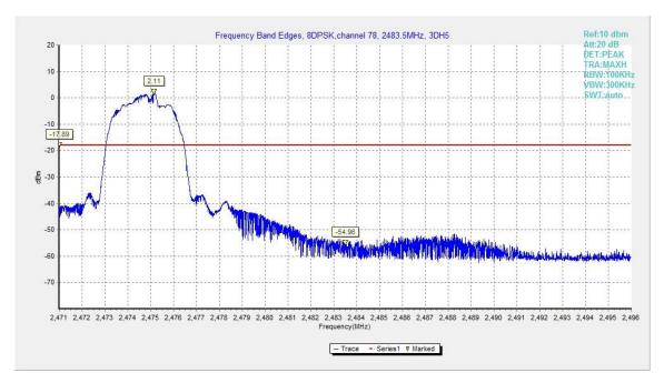
Fig.11. Frequency Band Edges: 8DPSK, Channel 78, Hopping Off
