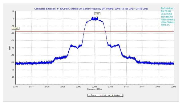
Fig.33. Conducted spurious emission:  $\pi/4$  DQPSK, Channel 39, 2441MHz
