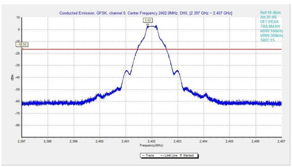
Fig.13. Conducted spurious emission: GFSK, Channel 0,2402MHz
