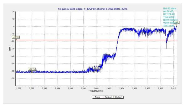
Fig.6. Frequency Band Edges: π/4 DQPSK, Channel 0, Hopping On
