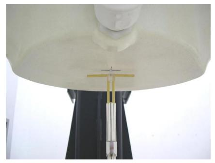
Picture 8.2 Photo of Dipole Setup
