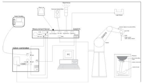
Picture C.1 SAR Lab Test Measurement Set-up
