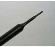
Picture C.2 Near-field Probe
