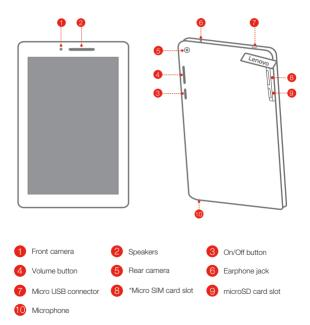
The WLAN model (Lenovo TB3-710F) does not have a Micro SIM card slot.
