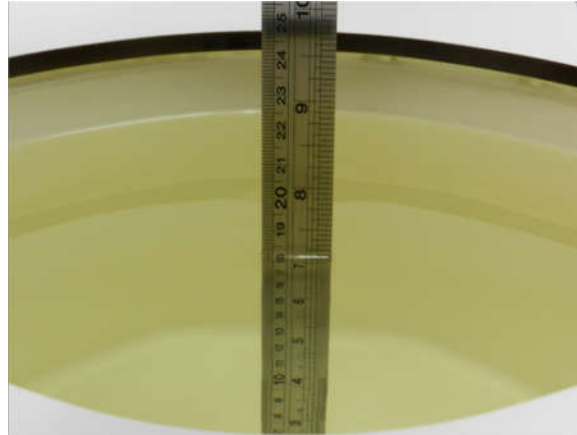
Fig 11.2 Photo of Liquid Height for Body SAR
