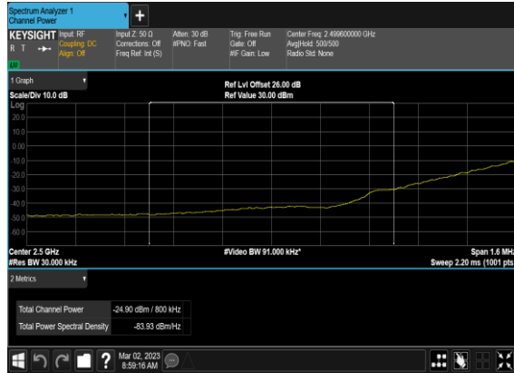
N7(40M)_DFT-s- OFDM_BPSK_Edge_1RB_Left_Low_CH_CHP_P ASS
