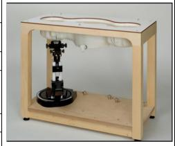
The shell corresponds to the specifications of the Specific Anthropomorphic Mannequin (SAM) phantom defined in IEEE 1528 and IEC 62209-1. It enables the dosimetric evaluation of left and right hand phone usage as well as body mounted usage at the flat phantom region. A cover prevents evaporation of the liquid. Reference markings on the phantom allow the complete setup of all predefined phantom positions and measurement grids by teaching three points with the robot.
