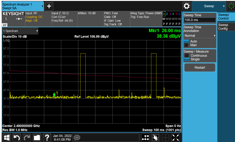
3DH5 on time (Count Pulses) Plot on Channel 39
