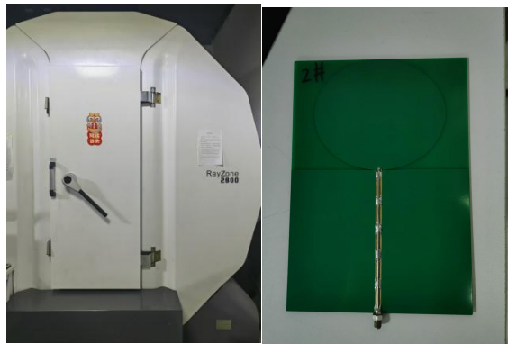
Fig 2 dipole model 3126-2500 frequency 2500 MHz
