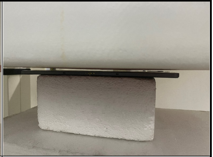
Rear Face of EUT with 0.5 cm Gap
