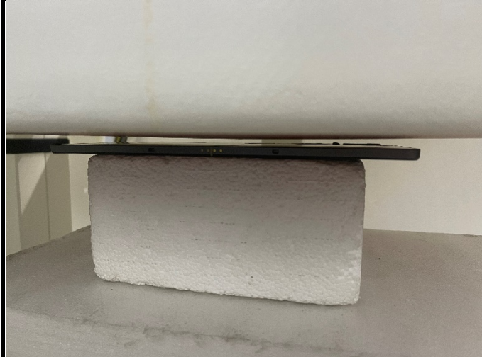
Rear Face of EUT with 0.7 cm Gap
