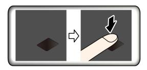
If the fingerprint reader indicator blinks in amber, the authentication is not successful.
