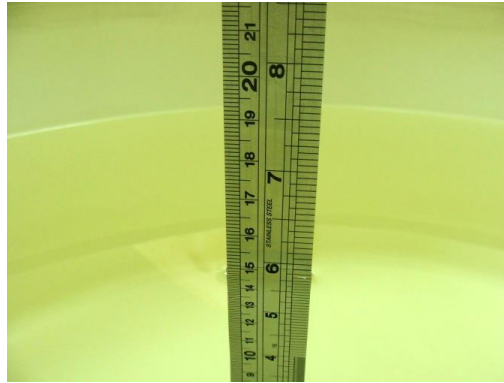
Fig 6.1 Photo of Liquid Height for Body SAR
