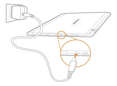
When the battery level falls below the threshold, IdeaTab will alert you with a tone and the battery status icon will change into 🔳 . We recommend you plug the AC power adapter into your IdeaTab in the direction of the orange arrow as shown above figure.
