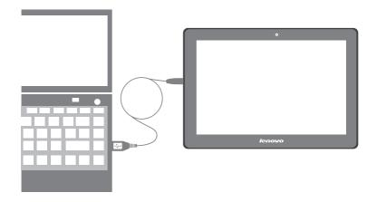
You can connect IdeaTab to the PC's USB port with the cable provided for battery charging or data transferring with the PC.
