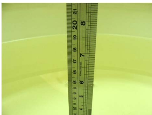
Fig 6.1 Photo of Liquid Height for Body SAR
