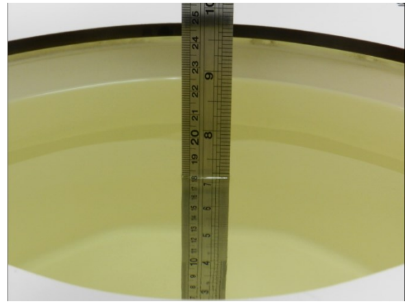
Fig 11.2 Photo of Liquid Height for Body SAR
