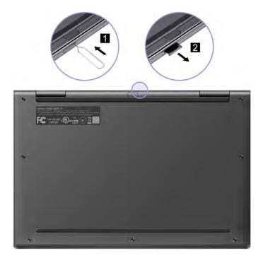
Step 2. Install a new nano SIM card into the tray and insert the tray into the nano SIM card slot. Ensure that the new nano SIM card is installed in the correct orientation.
