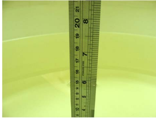
Fig 6.1 Photo of Liquid Height for Body SAR
