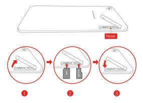
Step 1. Open the microSD card slot cover as shown.
