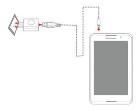
Method Connect your tablet to a power outlet using the included cable and USB power adapter.
