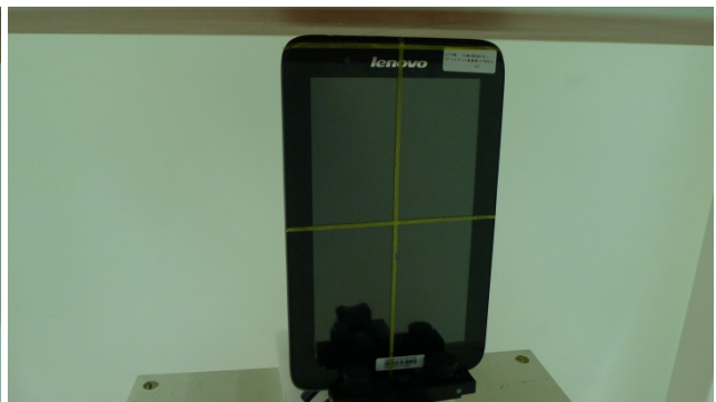
Edge1, Test Separation 0.4 cm
