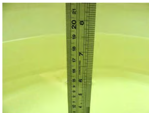
Fig 6.2 Photo of Liquid Height for Body SAR
