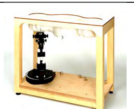
Fig 5.6 Photo of SAM Phantom
