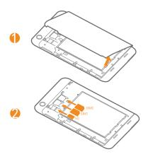
IdeaTab supports SD card and SIM card extension. To insert an SD card and SIM card , do the following:
