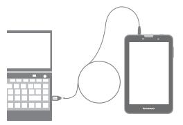
You can connect IdeaTab to the PC's USB port with the cable provided for battery charging or data transferring with the PC.
