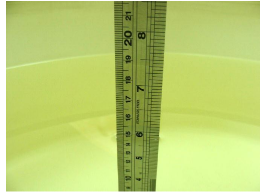
Fig 6.2 Photo of Liquid Height for Body SAR
