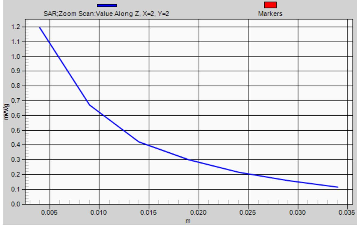
**#06 GSM850\_GPRS12\_Bottom Face\_0cm\_sensor on\_Ch128**
