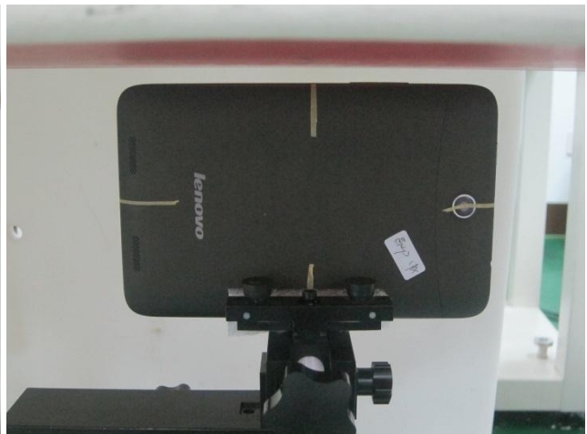
Primary Portrait of the DUT with Phantom 0.7 cm Gap
