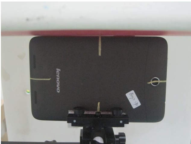
Primary Portrait of the DUT with Phantom 0 cm Gap
