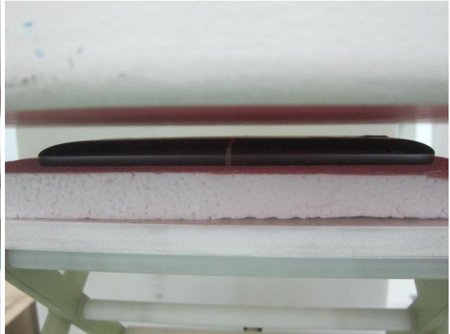
Bottom Face of the DUT with Phantom 0.9 cm Gap
