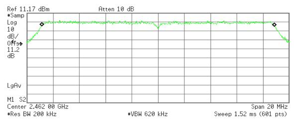
Occupied Bandwidth 17.7501 MHz Occ BW % Pwr 99.00 % x dB -26.00 dB
