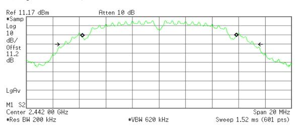
Occupied Bandwidth 11.5785 MHz Occ BW % Pwr 99.00 % x dB -26.00 dB
