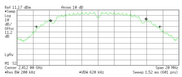
Occupied Bandwidth 11.7636 MHz Occ BW % Pwr 99.00 % x dB -26.00 dB
