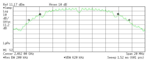
Occupied Bandwidth 11.8070 MHz Occ BW % Pwr 99.00 % x dB -26.00 dB
