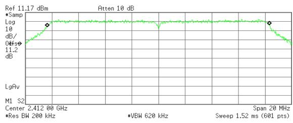
Occupied Bandwidth 16.7137 MHz Occ BW % Pwr 99.00 % × dB -26.00 dB
