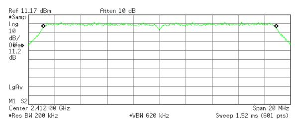
Occupied Bandwidth 17.7557 MHz Occ BW % Pwr 99.00 % x dB -26.00 dB
