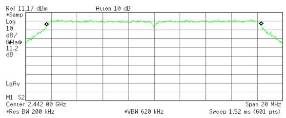
Occupied Bandwidth 16.7003 MHz Occ BW % Pwr 99.00 % x dB -26.00 dB
