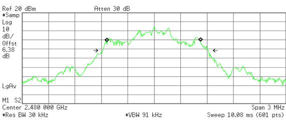
Occupied Bandwidth 1.0586 MHz Occ BW % Pwr 99.00 % **x dB** -26.00 dB
