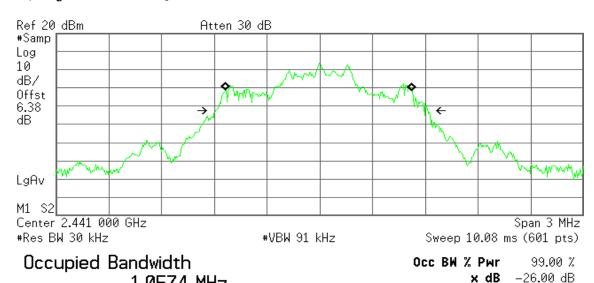
Transmit Freg Error -6.439 kHz x dB Bandwidth 1.205 MHz\*
