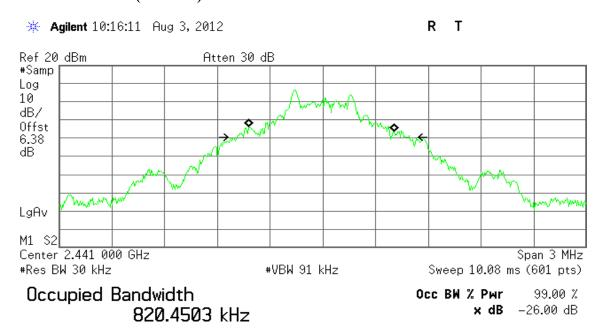
Transmit Freq Error -7.534 kHz x dB Bandwidth 979.347 kHz\*
