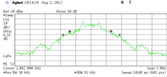
Occupied Bandwidth 810.4784 kHz Occ BW % Pwr 99.00 % x dB -26.00 dB
