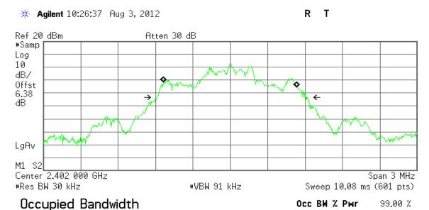
Transmit Freq Error -4.143 kHz x dB Bandwidth 1.206 MHz\*
