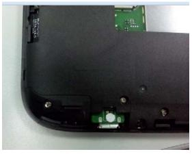
Except for the antenna shape changes listed above, and adding absorbing material beside BT/WIFI antenna, antenna type, material and the gain of antenna and matching are in all relevant parts identical to the original product.
