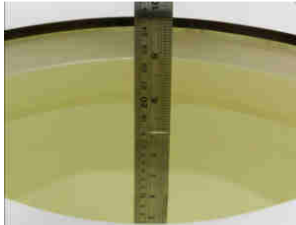
Fig 10.1 Photo of Liquid Height for Body SAR
