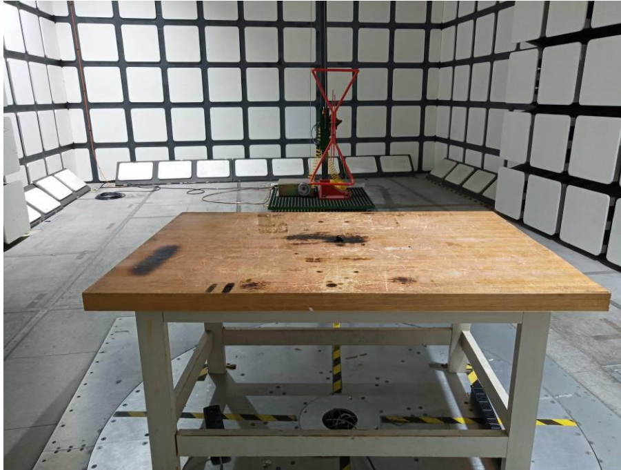
Radiated Emissions View (Below 1 GHz)
