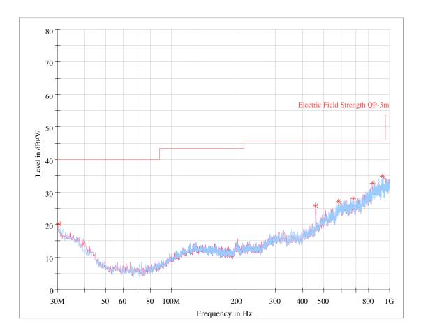
**30 MHz~1 GHz:** (the worst case is 8DPSK Mode, Low channel)
