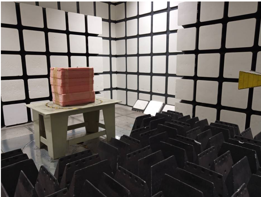
Radiated Emissions View (Above 1 GHz)
