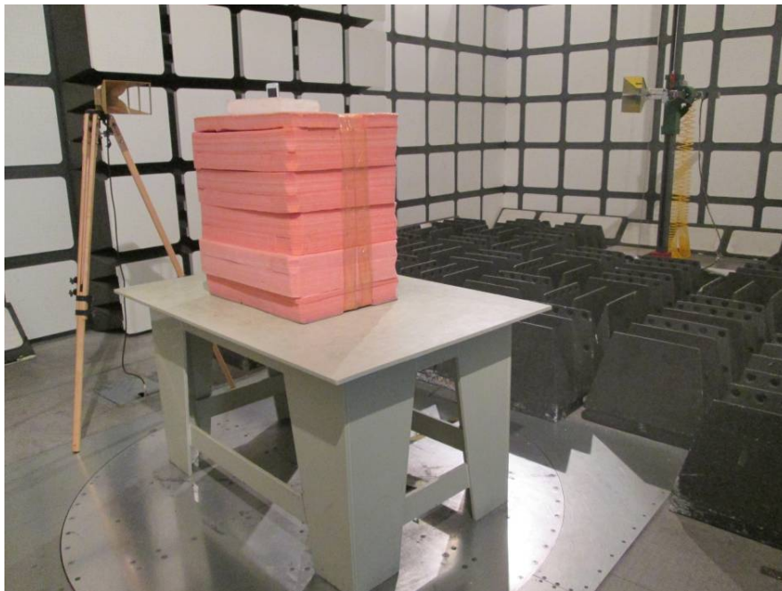
Radiated Emissions Test View (Above 1 GHz)
