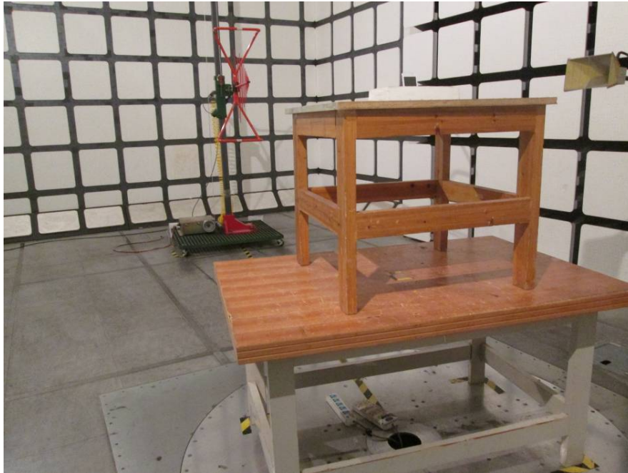
Radiated Emissions Test View (Below 1 GHz)
