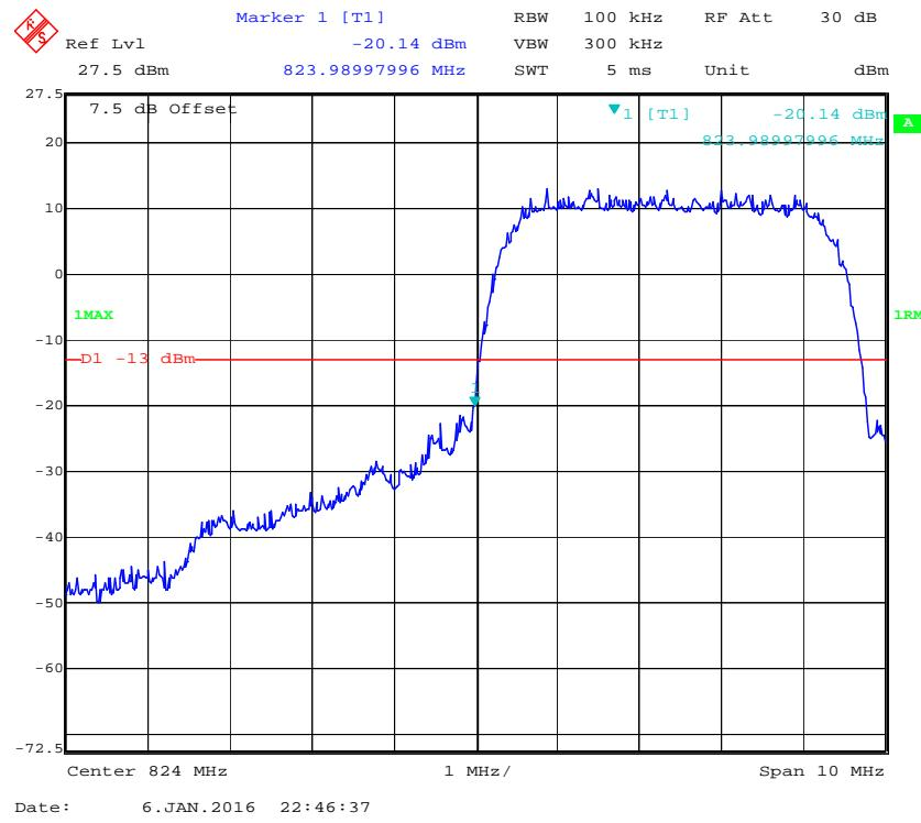
**Cellular Band, Right Band Edge for HSDPA (16QAM) Mode**
