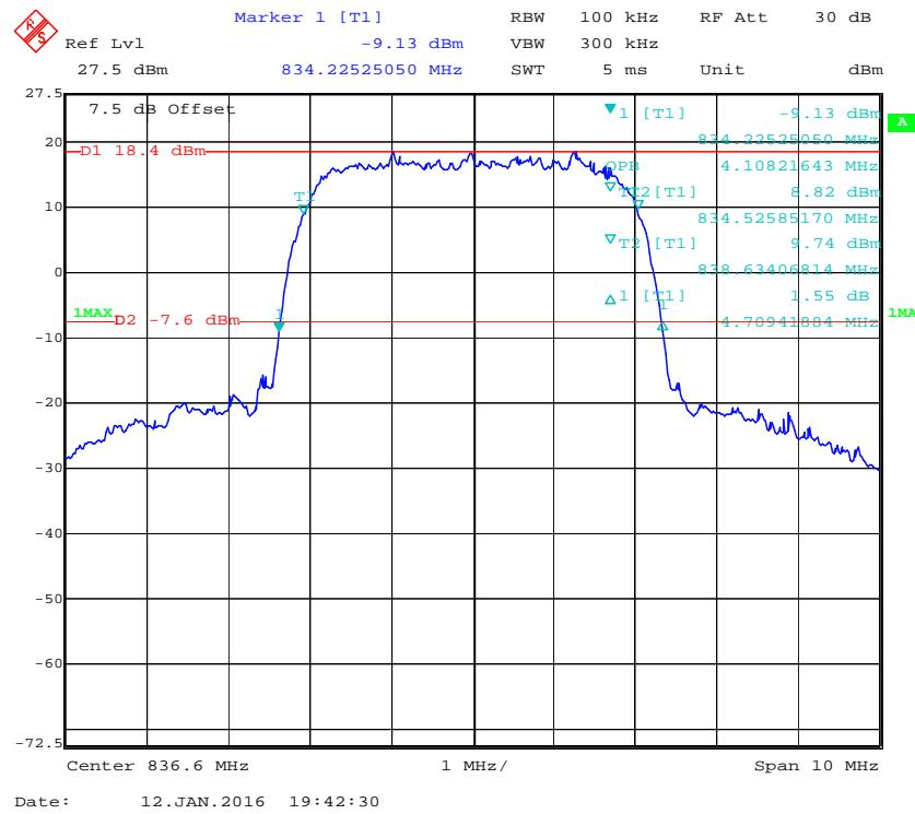
**PCS Band (Part 24E)****99% & 26 dB Occupied Bandwidth for GSM (GMSK) Mode**
