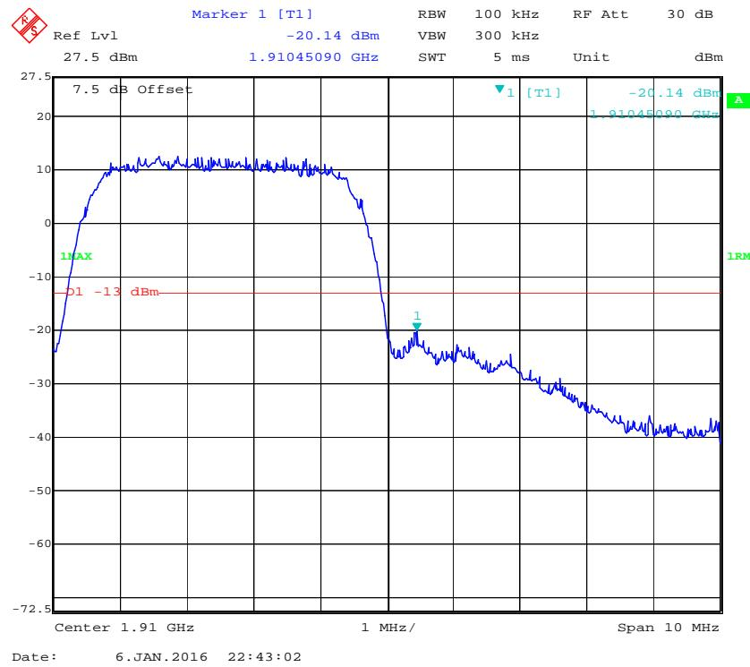
**PCS Band, Left Band Edge for HSDPA (16QAM) Mode**
