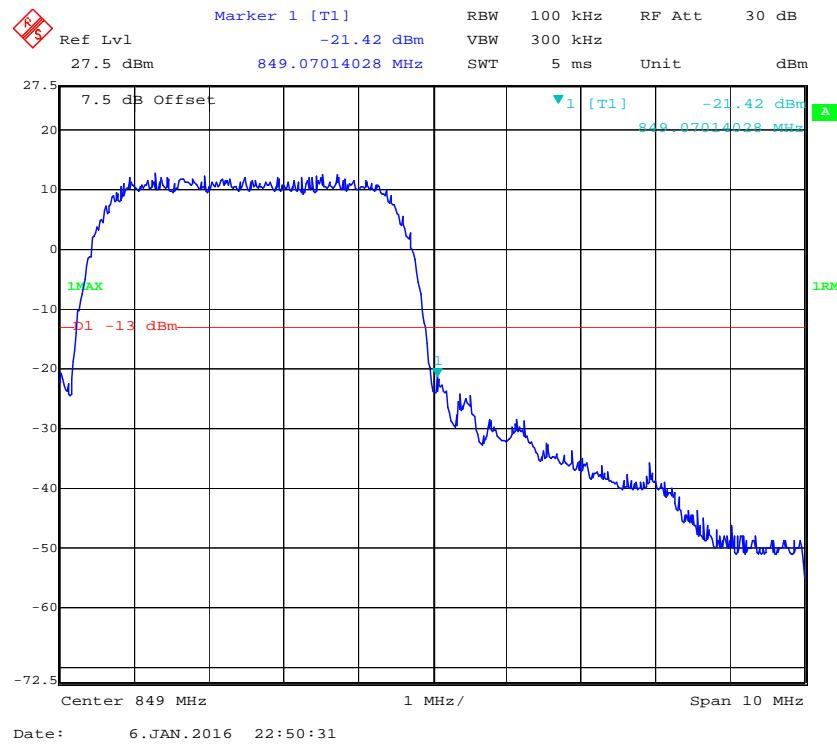
**Cellular Band, Left Band Edge for HSUPA (BPSK) Mode**
