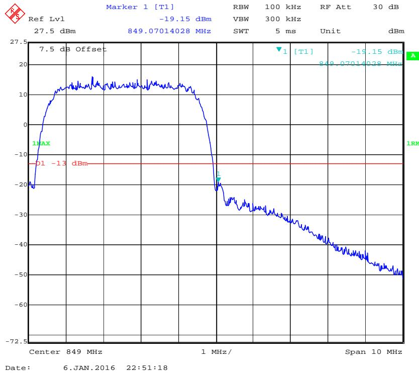
**Cellular Band, Left Band Edge for HSDPA (16QAM) Mode**
