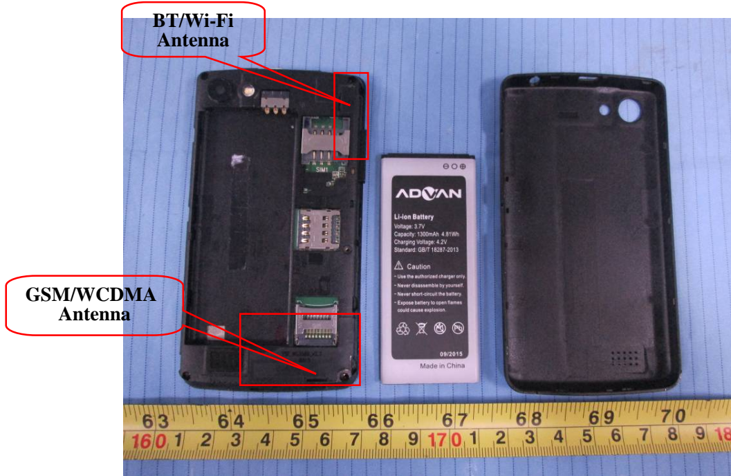
EUT –Cover off View 1
