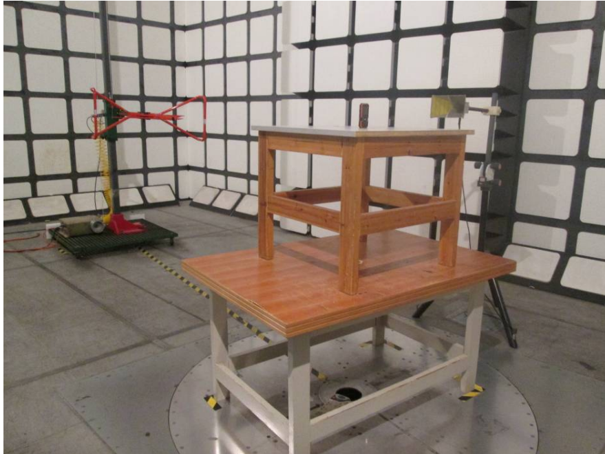
Radiated Emissions Test View (Below 1 GHz)
