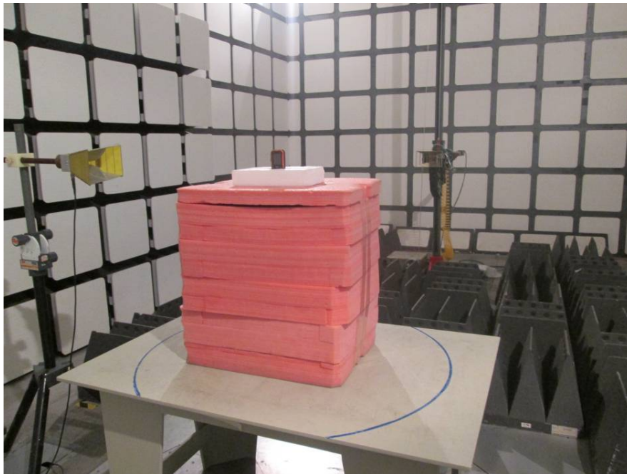
Radiated Emissions Test View (Above 1 GHz)
