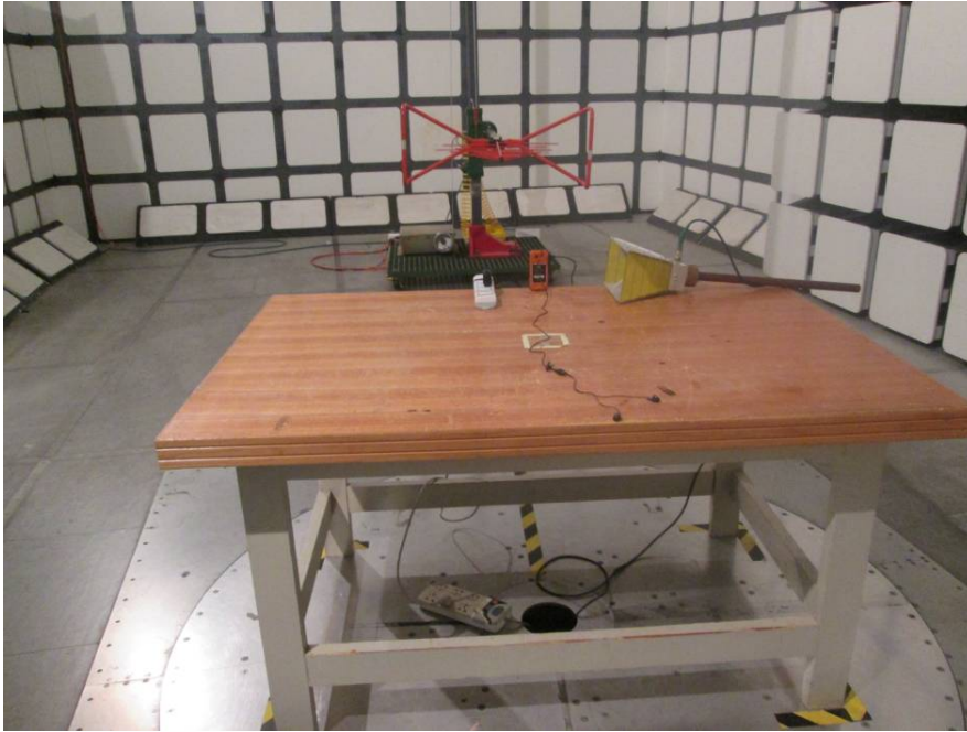
Radiated Emissions Front View (30-1000 MHz)
