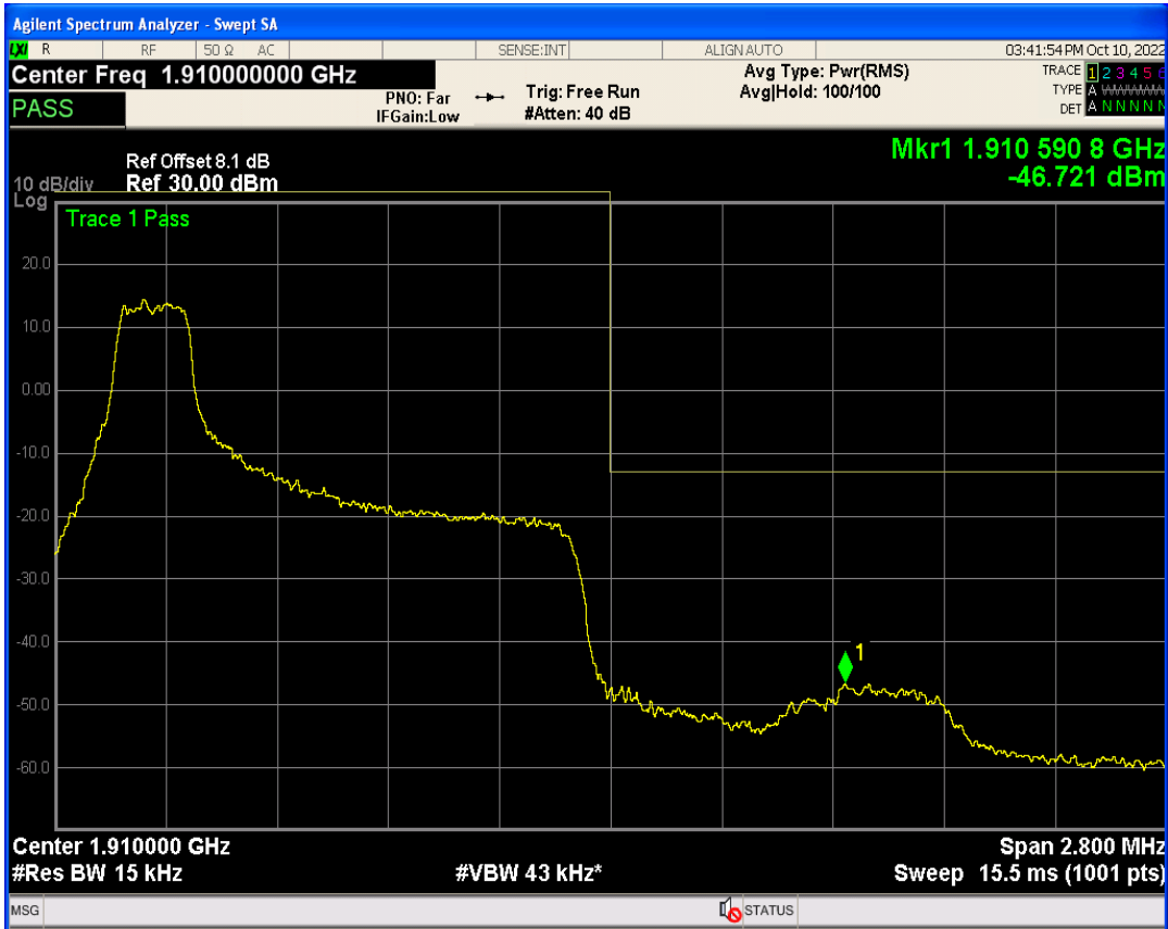
Band2 QPSK BW=1.4MHz Channel=19193 RB Size=1 Position=#Max
