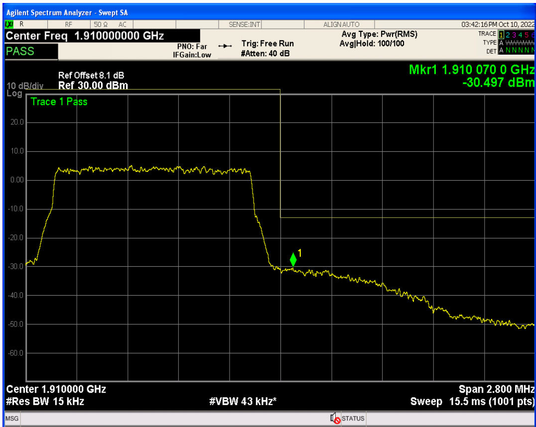
Band2 QPSK BW=3MHz Channel=18615 RB Size=1 Position=#Max
