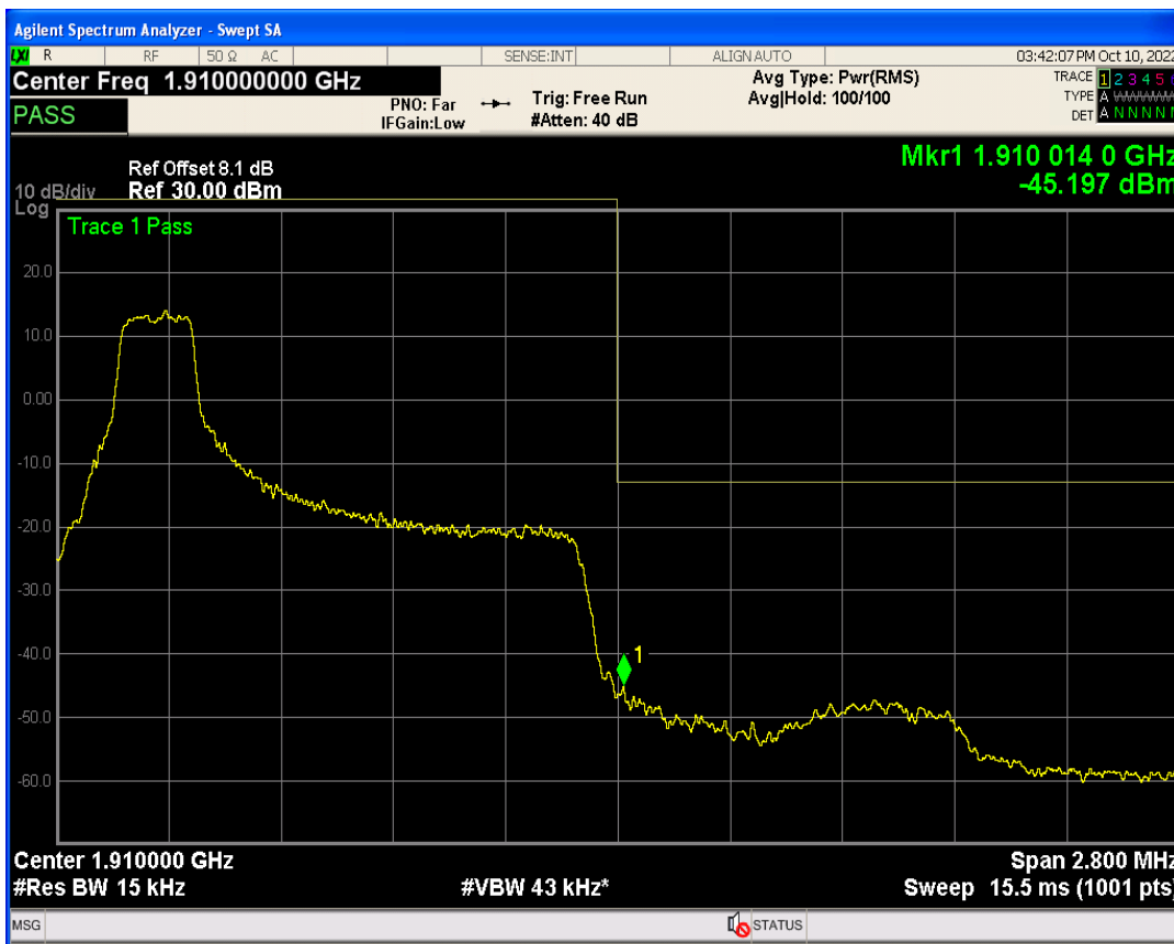
Band2 QPSK BW=1.4MHz Channel=19193 RB Size=6 Position=#0
