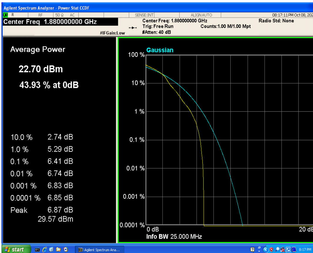
Band2 QPSK BW=20MHz Channel=18900 RB Size=1 Position=#0
