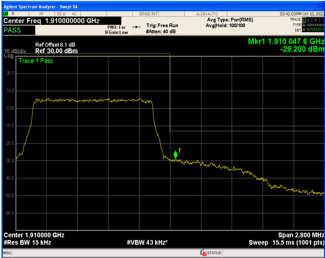
Band2 QAM16 BW=1.4MHz Channel=19193 RB Size=1 Position=#Max
