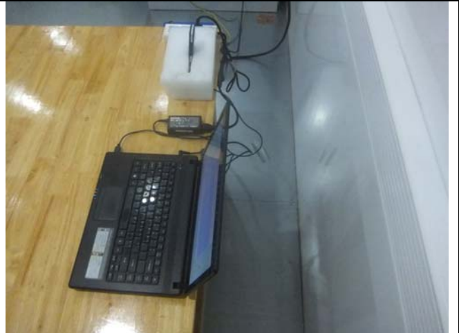
Conducted Emissions Test Setup – Side View
