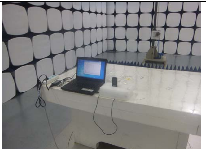
Radiated Spurious Emissions Test Setup Above 1GHz
