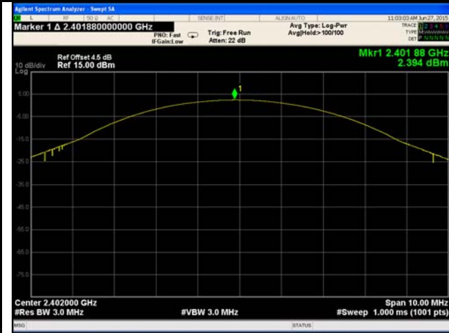
8DPSK Output power - Low CH 2402
