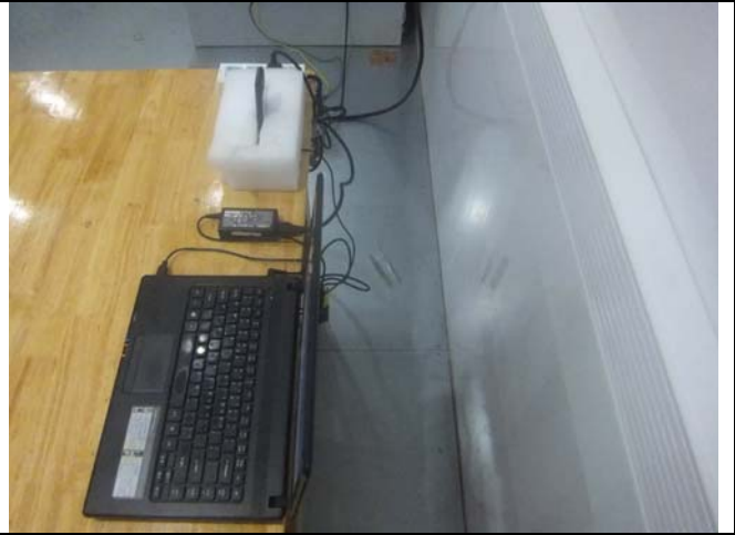
Conducted Emissions Test Setup – Side View
