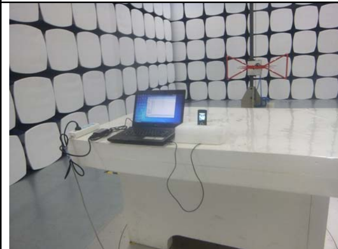
Conducted Emissions Test Setup – Front View
