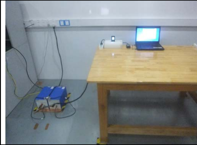
Conducted Emissions Test Setup – Front View
