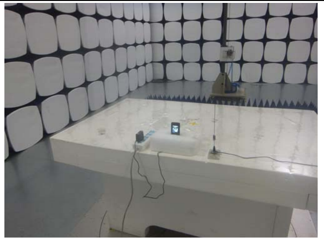
Radiated Spurious Emissions Test Setup Above 1GHz
