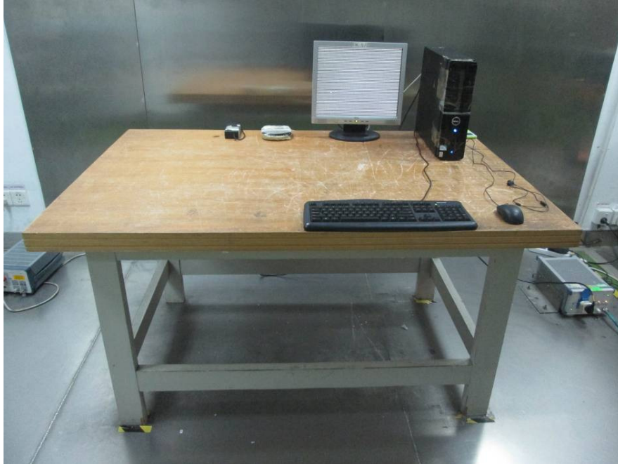
Conducted Emissions - Front View (Downloading)
