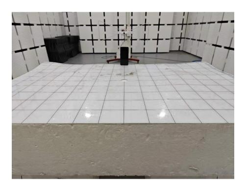
Set-up for Radiated Spurious Emission, Above 1GHz
