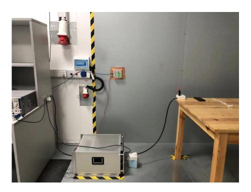
Set-up for Radiated Emission (RE), Below 1GHz
